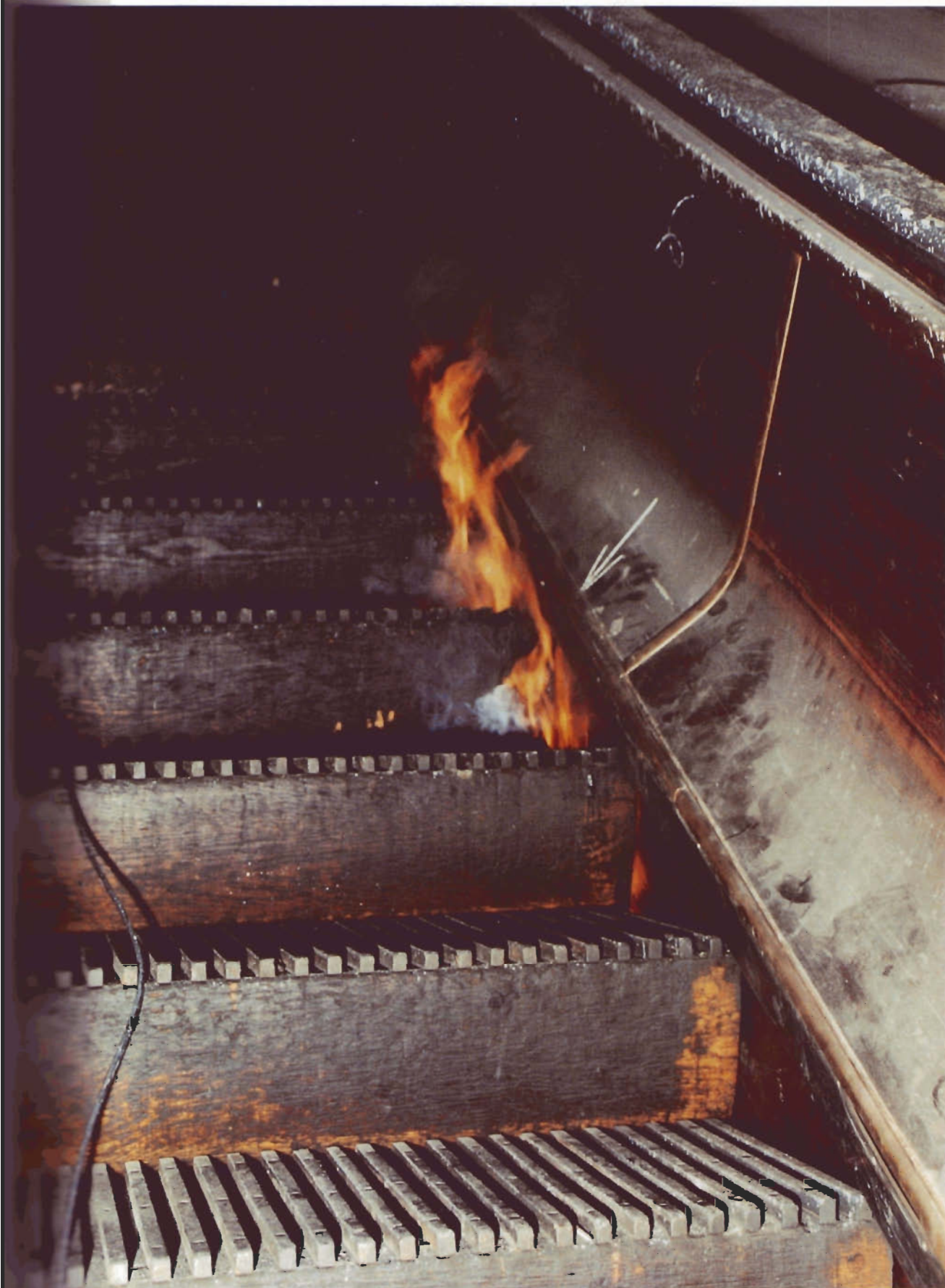
23 Fire development trials on escalator 4 on 8 January 1988, 8 minutes 41 seconds after application of lighted match. Arrow indicates entry of match
