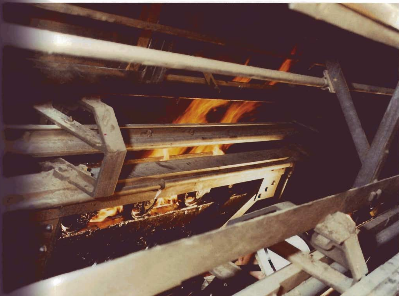
Fire development trials on escalator 4 on 8 January 1988, 7 minutes and 11 seconds after application of lighted match, viewed from beneath
