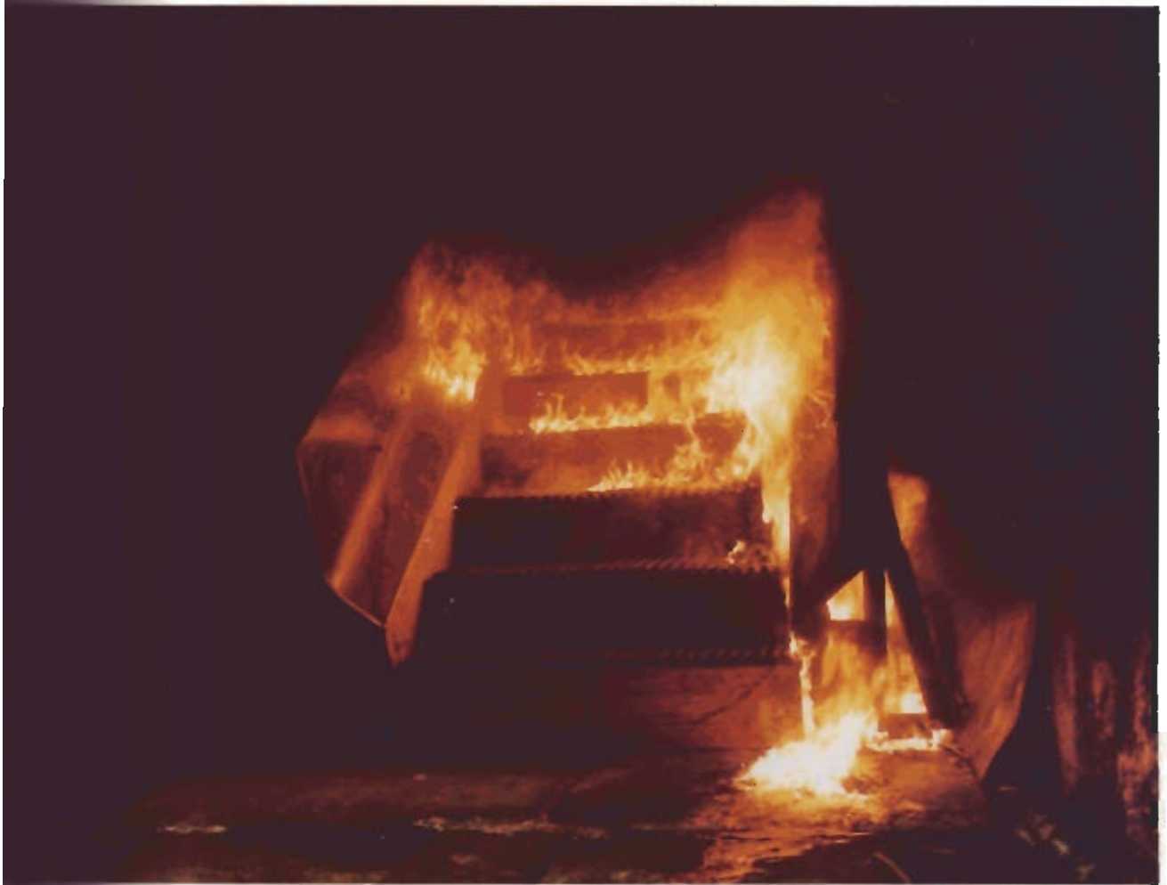
Fire test on six full-scale steps of an escalator at the Health and Safety Executive, Buxton
